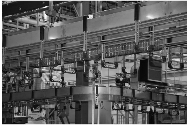
Fig. 7.5 The air conveyor system for the transport of PET bottles between blow-moulding machine and filler.
