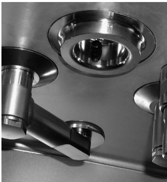
Fig. 7.24 Automated CIP cups close the filling valves to create a cleaning loop.
