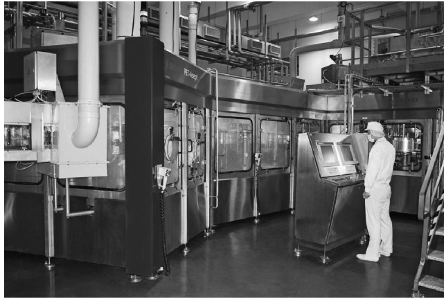
Fig. 7.19 In an aseptic filling concept, the filler and its systems are completely separated from their surroundings.
