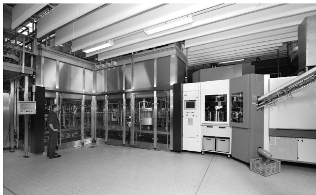
Fig. 7.6 Preforms are delivered on the right to the heating oven. The blow-moulding process can be observed via the windows in the blow-moulding machine. The filling system is also directly blocked (from the middle to the left) with a hygienic housing and a fully automated filling procedure.
