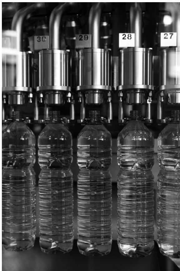
Fig. 7.20 In the hygienic filling design, the bottle is filled without any contact with the filling valve.
