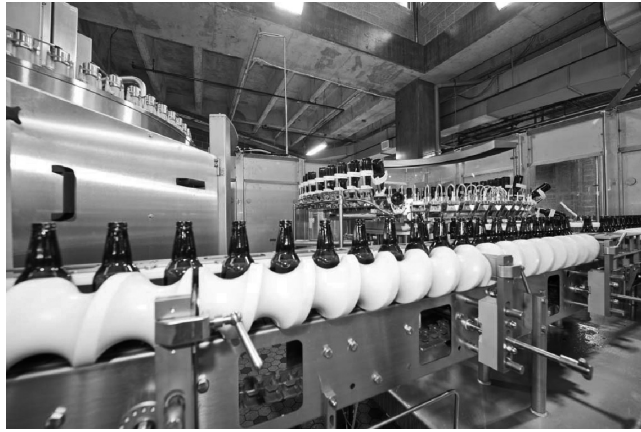
Fig. 7.16 Infeed worm separating the bottles to match them to the pitch of the filler.
